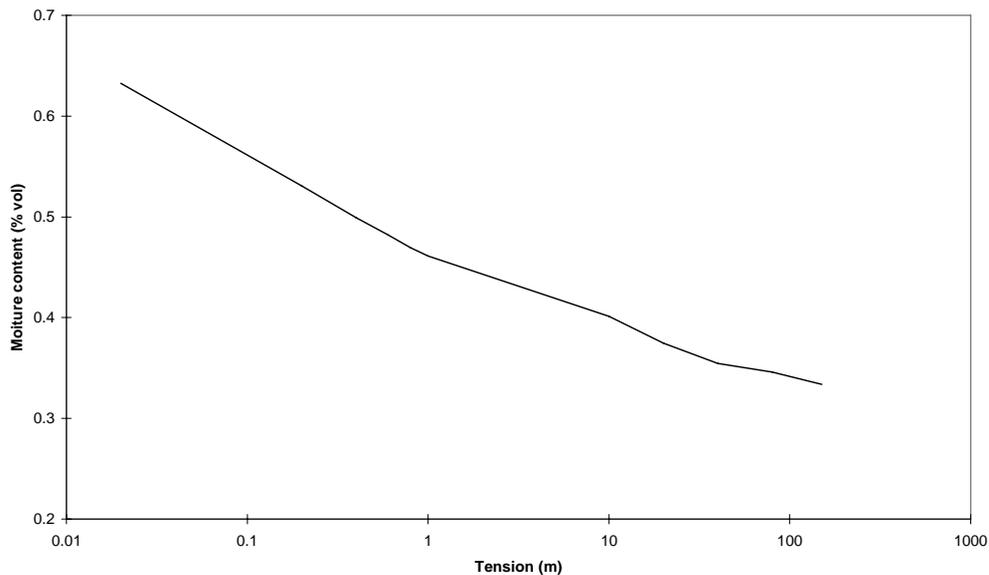
Figure 6.16 Soil moisture release curve for Blackthorn Meadow IV topsoil
