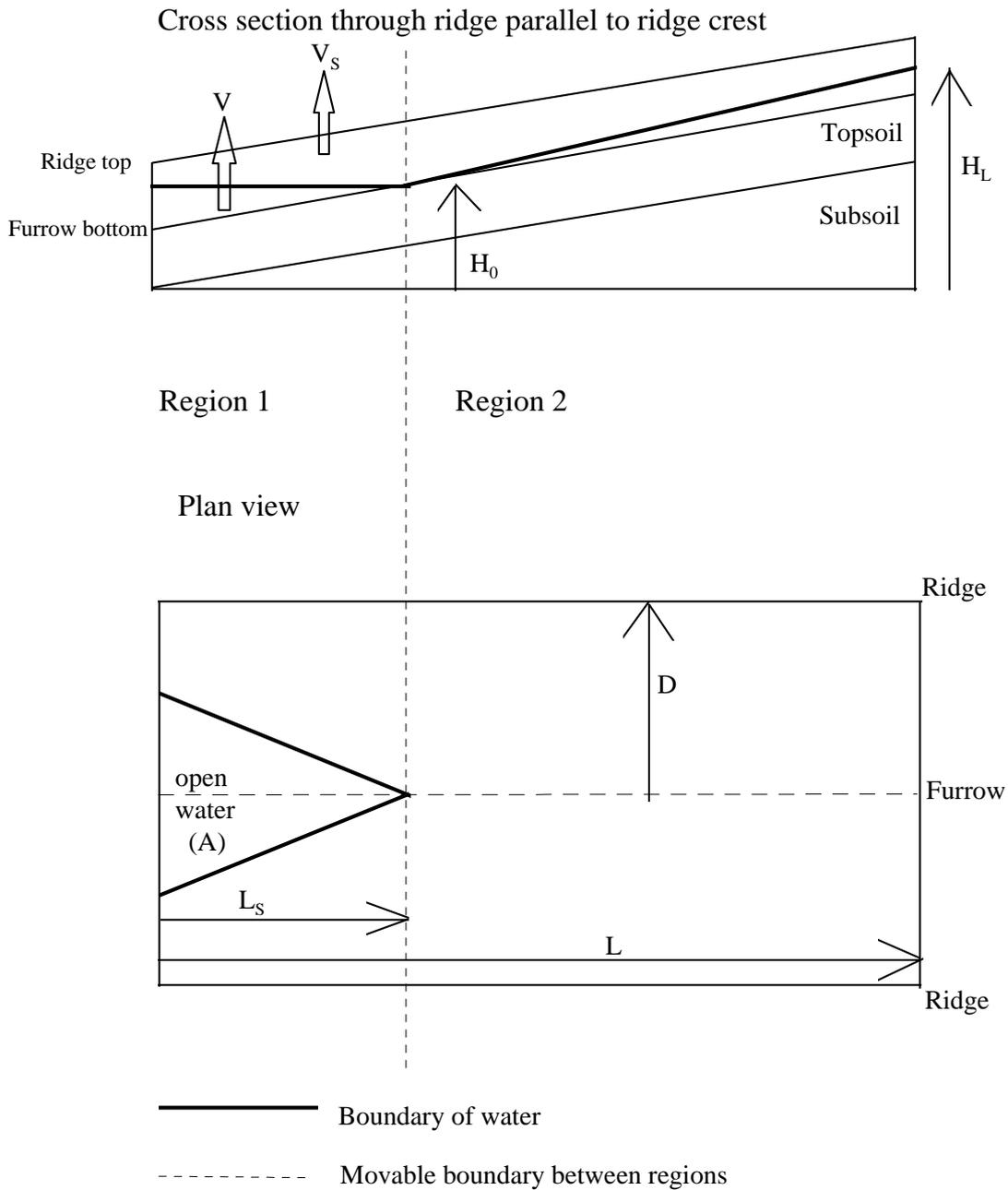
Figure 6.11      Diagram to show the boundaries used in the ridge and furrow water-balance model.
