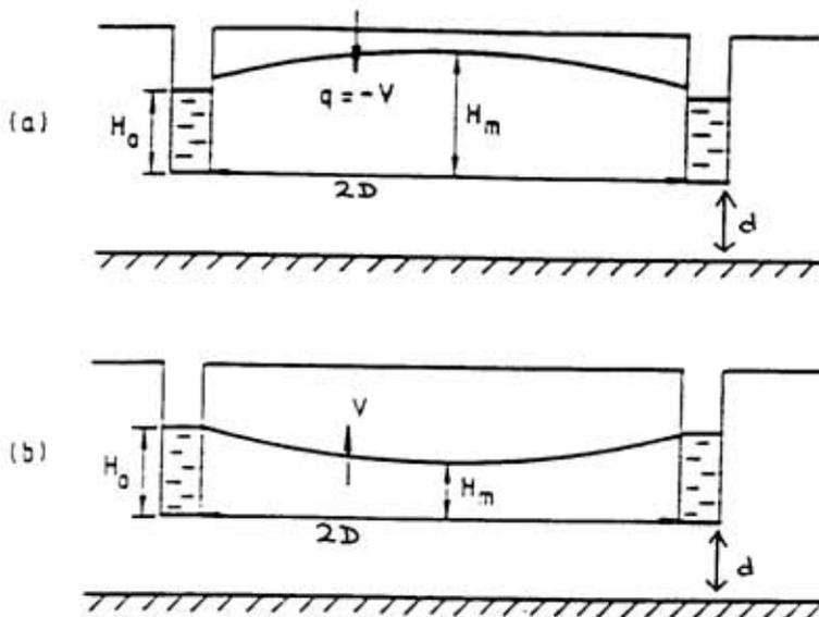
Figure 6.2 The water-table shape between water-filled ditches acting as drains (a) and as irrigation channels (b)
