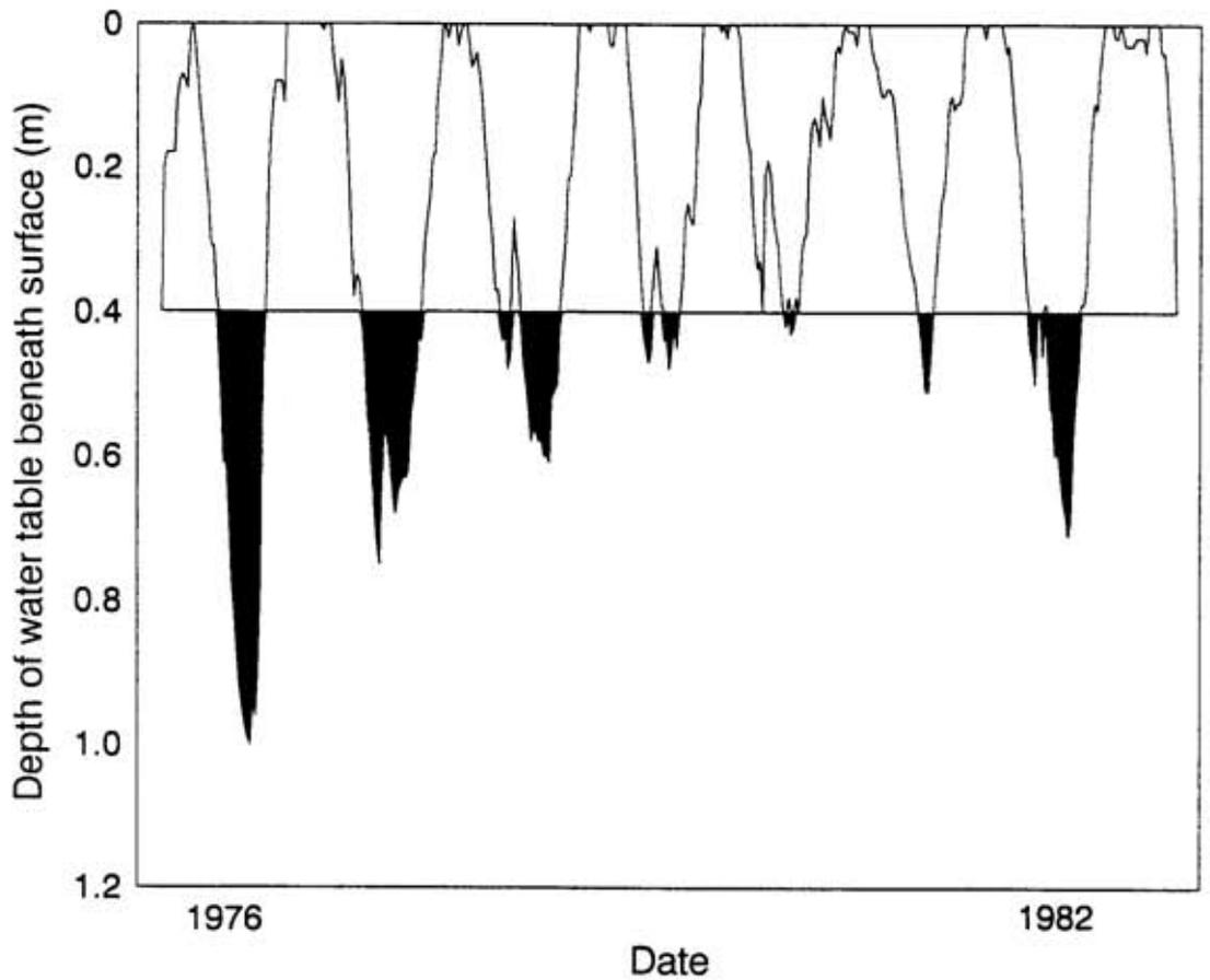
Figure 6.15 Hydrograph over a 7-year period demonstrating the between-year variation in SEVs due to fluctuation in rainfall amounts and patterns.
