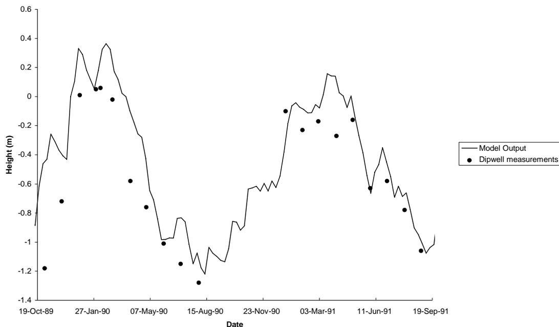
Figure 6.10 Model output shown against dipwell measurements for Cricklade North Meadow
