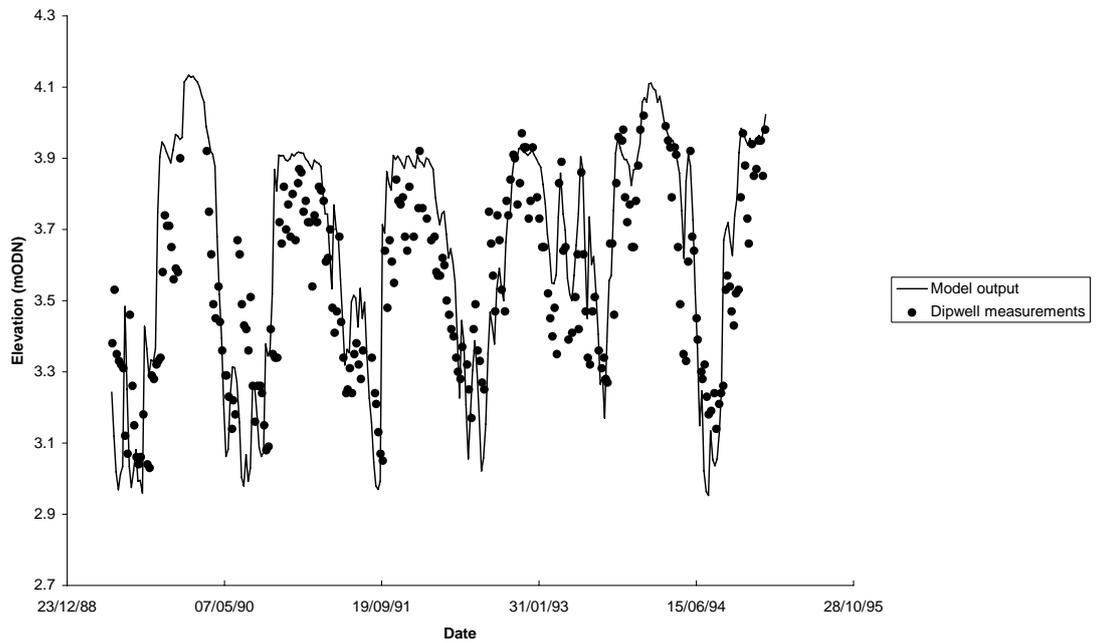
Figure 6.6 Model output shown against dipwell measurements for Southlake Moor
