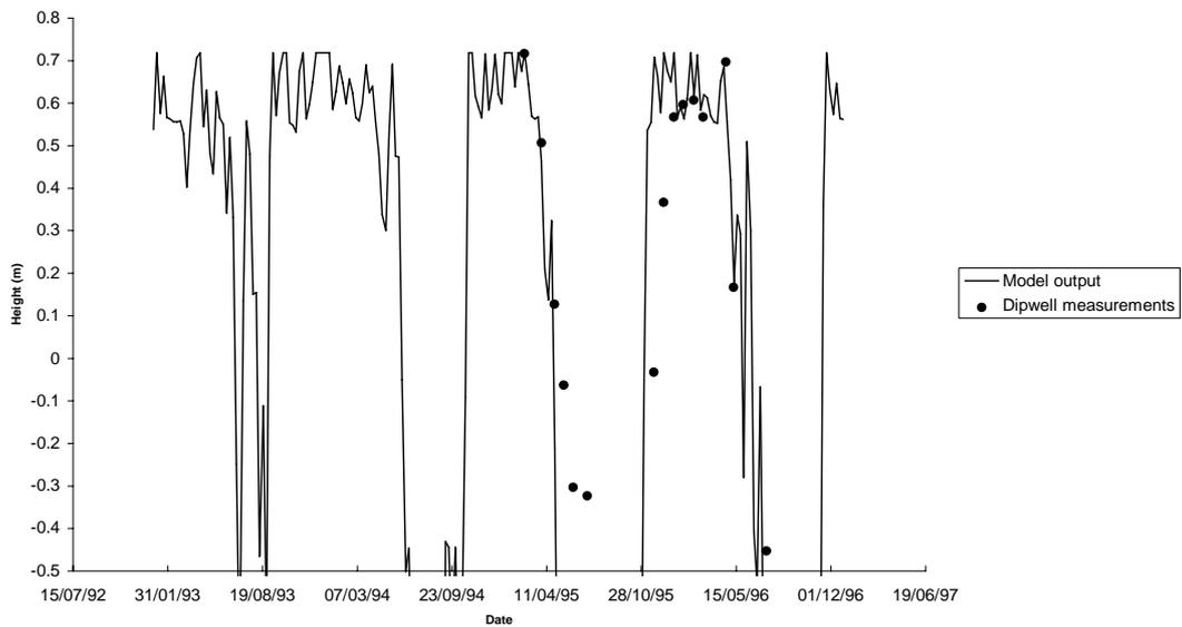
Figure 6.13 Model output shown against dipwell measurements for Blackthorn Meadow IV. Height relative to an arbitrary datum.
