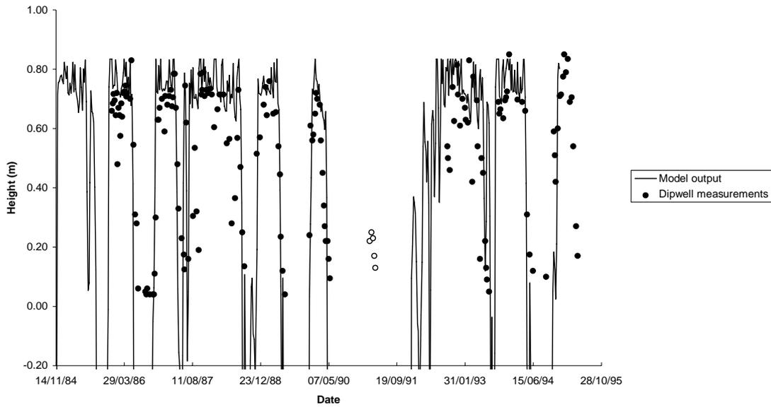
Figure 6.12 Model output shown against dipwell measurements for Upwood Meadows. Height relative to an arbitrary datum (The hollow circles represent water perched in the dipwell that was assumed to be unconnected to a true water table. This situation occurred following an exceptionally dry summer.)
