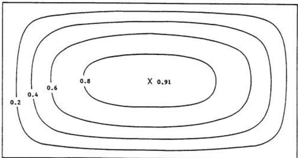
Figure 6.1 Contours of seepage potential (shape factors) for a rectangular field with one side twice the length of the other.
