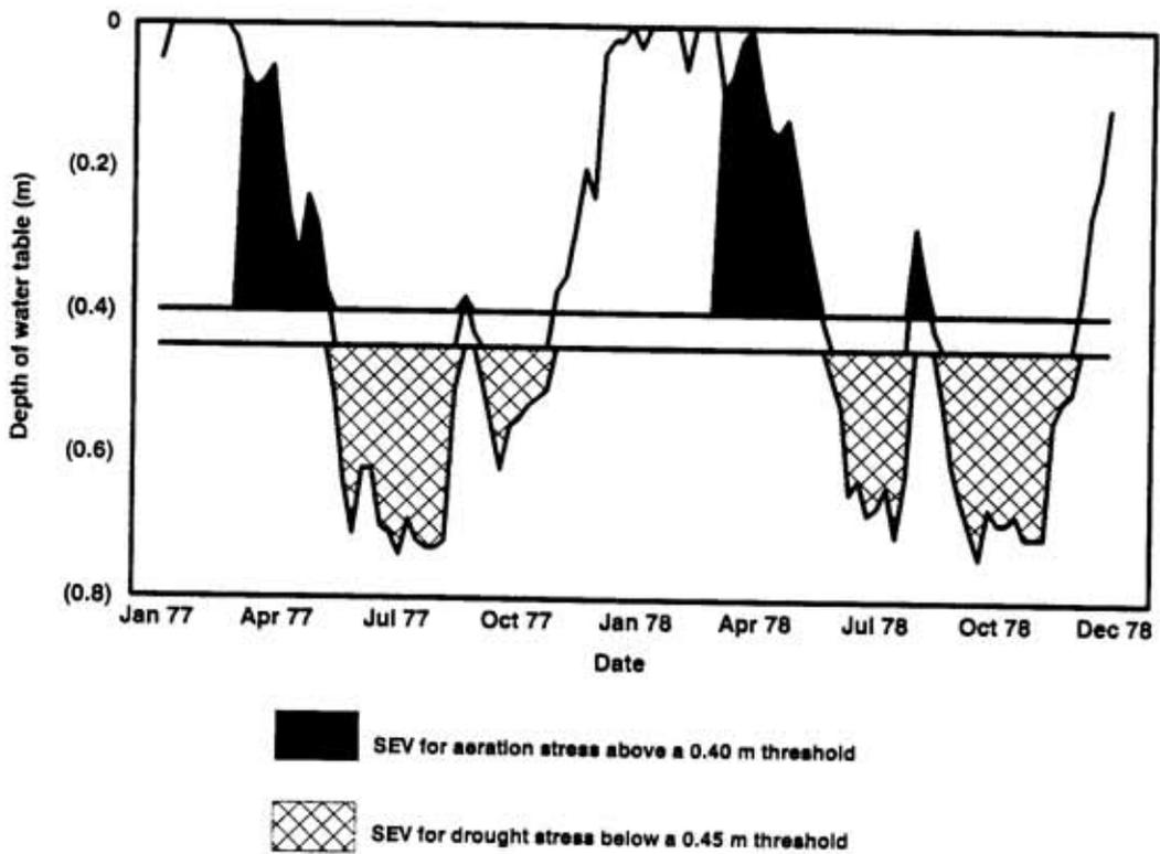
Figure 6.14 A hydrograph showing water-table depth variation over two annual cycles. The shading illustrates how Sum Exceedence Values are derived.
