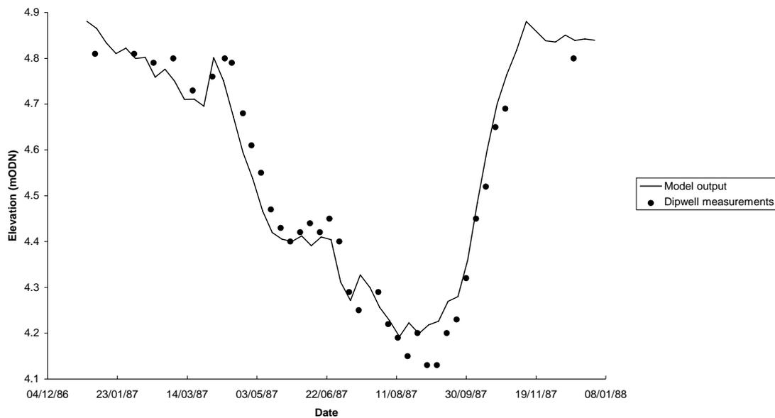
Figure 6.4 Model output shown against dipwell measurements for West Sedgemoor
