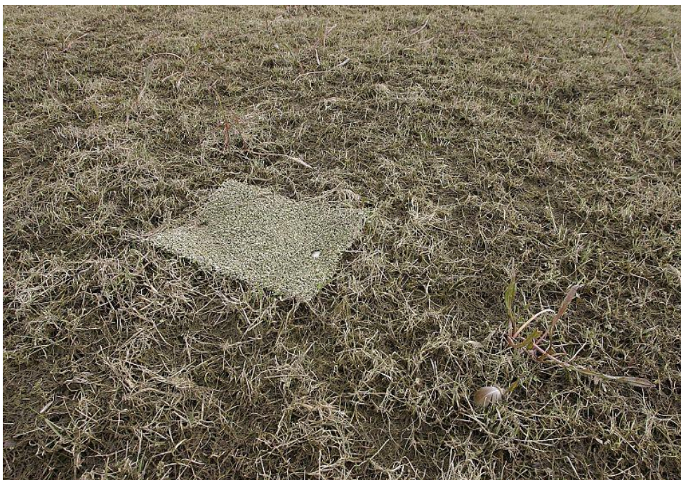
Small pieces of astro turf (weighed in advance and pinned down with pegs), called 'sedimats' are used to capture sediment deposited during a flood. They must be placed on site before a flood and then collected and removed to a lab
